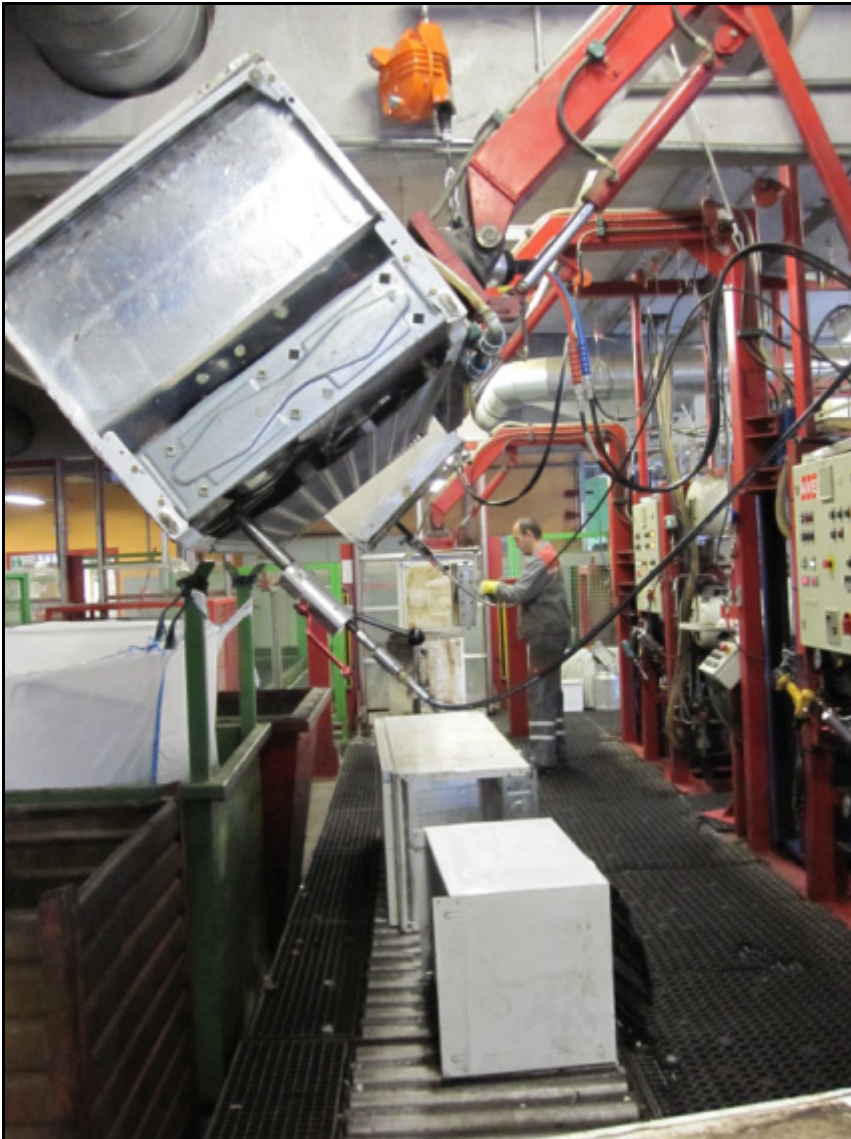
Picture 15 Step 1 of CFC recovery from refrigerators
