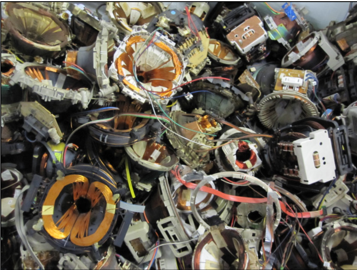
Picture 13 Focusing and deflecting coils of manually dismantled CRTs (Source: Öko-Institut 2010)
